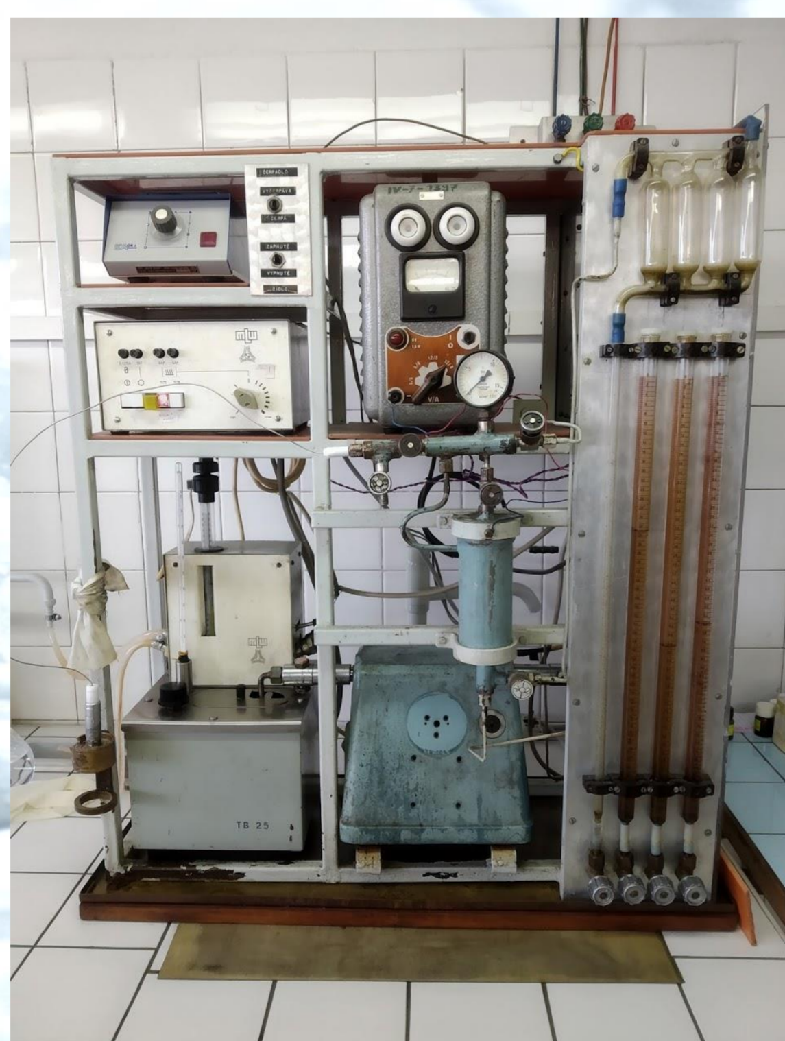
Fig.2 Reactor: glass-lined stainless steel with monitoring of the oxygen consumption
