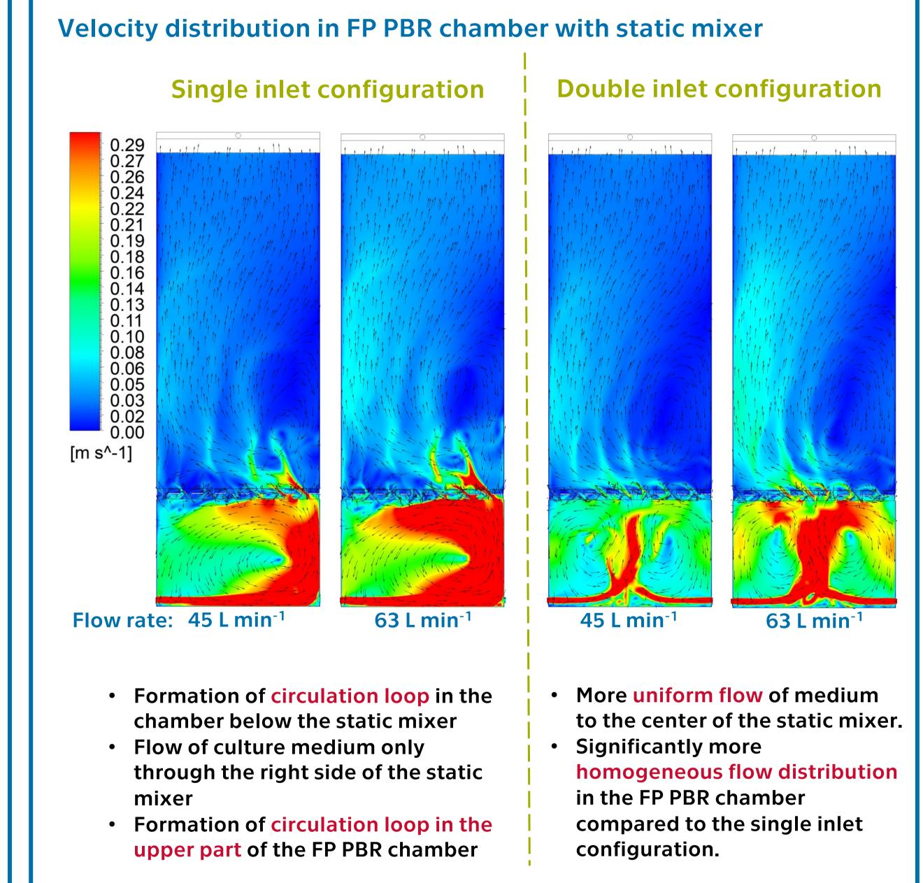
Based on the measurement, it can be determined that the measured and simulated streamlines were in a good agreement and the CFD model can be used to simulate various operating conditions in FP PBR with an installed static mixer.
