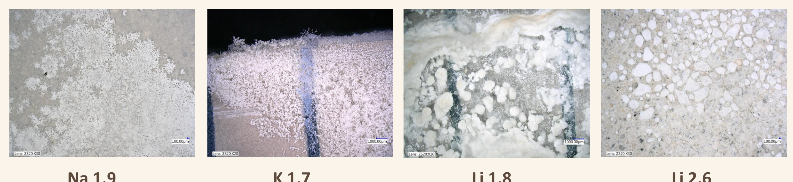
Fig. 7: Detailed photos of efflorescence taken by microscopy method.
