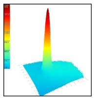
highest microlenses (h  $\approx$  2,2 µm) were obtained on the surface of glass with 59 mol % of GeS<sub>2</sub>. From the dependence of the microlenses height on the radiation intensity the threshold value of microlens formation was determined. This value indicates the minimal energy for surface changes/microlenses formation.
