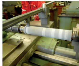
Figure 8. Measurement of the abrasive resistance of cylindrical corundum coatings with a thickness of 230 \mu\text{m}
