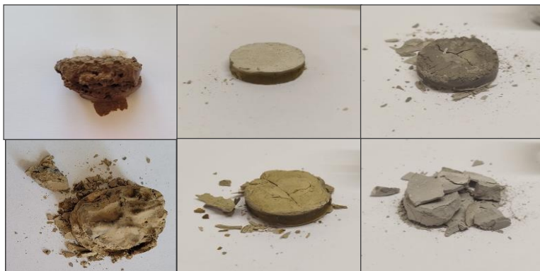
Figure 6. The mineralised WCF samples (Gutter, Highway, and Column from left to right; top row — samples mineralised by S. pasteurii DSM 33; bottom row — mineralised by S. jiandibaonis U2)
