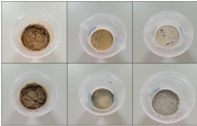
Figure 4. The WCF samples mineralised by S. jiandibaonis U2 (Gutter, Highway, and Column from left to right; top row — samples with 2x addition of bacteria; bottom row — only initial addition of bacteria)
