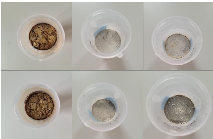
Figure 5. The WCF samples mineralised by S. pasteurii DSM 33 (Gutter, Highway, and Column from left to right; top row — samples with 2x addition of bacteria; bottom row — only initial addition of bacteria)
