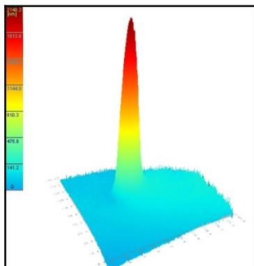
highest microlenses ( $h \approx 2,2\ \mu\text{m}$ ) were obtained on the surface of glass with 59 mol % of  $\text{GeS}_2$ . From the dependence of the microlenses height on the radiation intensity the threshold value of microlens formation was determined. This value indicates the minimal energy for surface changes/microlenses formation.
