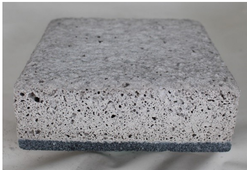
Figure 1 Composite block prepared from cast geopolymer and pressed geopolymer board.
